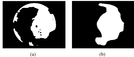
Fig. 2. (a) Segmentation by SVM with only average saturation as input, (b) ground truth
