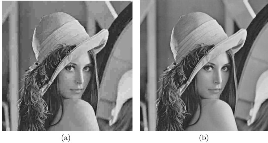
Fig. 2. Decompressed image by (a) Q_{10} and (b) quantization table Q_{10\_opt} obtained by gFWA
