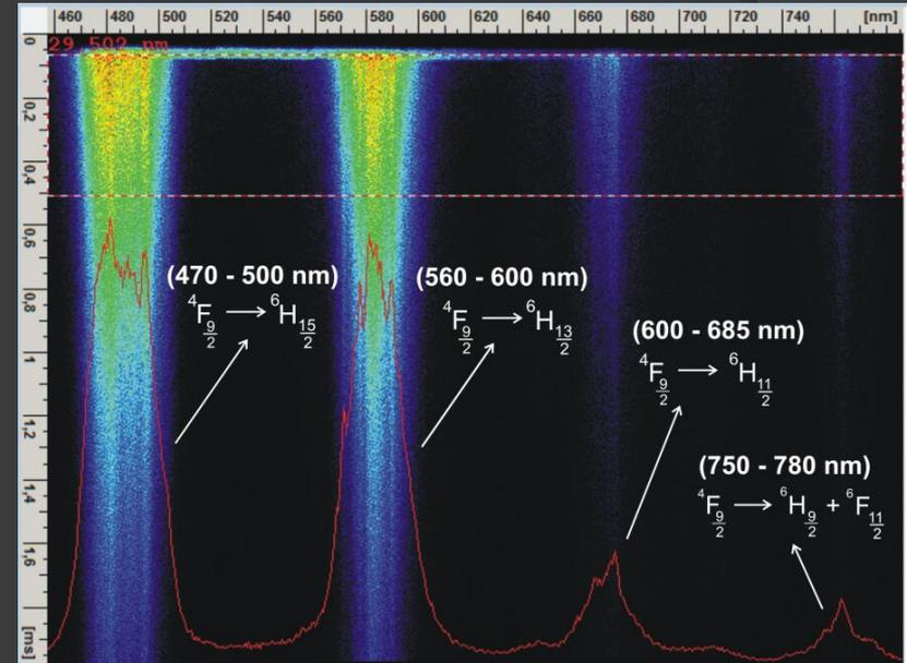
Time-resolved photoluminescence spectrum of  $\text{Dy}^{3+}$  dopanega YAG nanopowder
