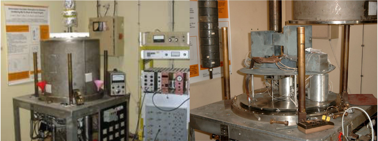
Figure 2. Photos of electron spectrometer ESMA at the IPB showing vacuum chamber and electronics as well as the inside vacuum chamber
