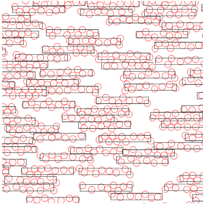
Figure 14. Typical jammed-state configuration of a region of size 30 \times 30 (in units of the disk diameter d_0 ,) for \theta_0^{(\text{cell})} = 0.45 . Orientation of rectangular cells with sides \alpha = 8 and \beta = 1 is fixed to the horizontal direction.
